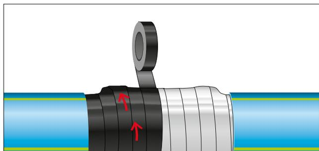
6.79 Wrap GEROfit® sealing tape around the joint
