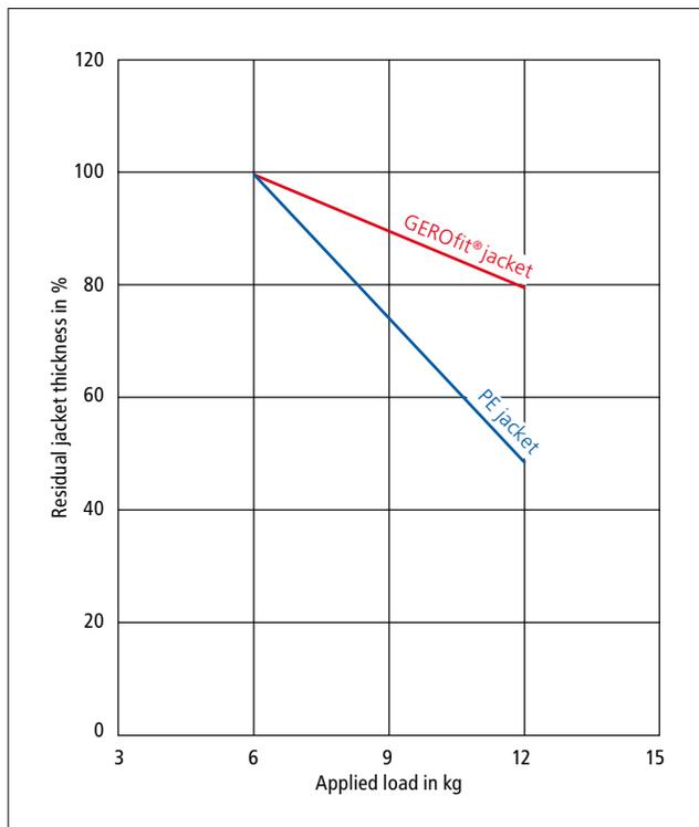
6.14 Scratch test comparison between GEROfit® and PE jackets acc. to PAS 1075
