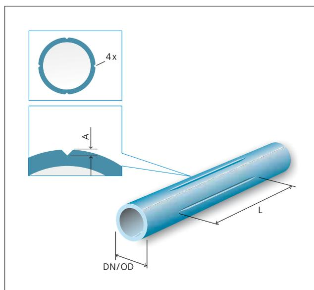
6.8 NPT – Notched pipe test (acc. to ISO 13479)
