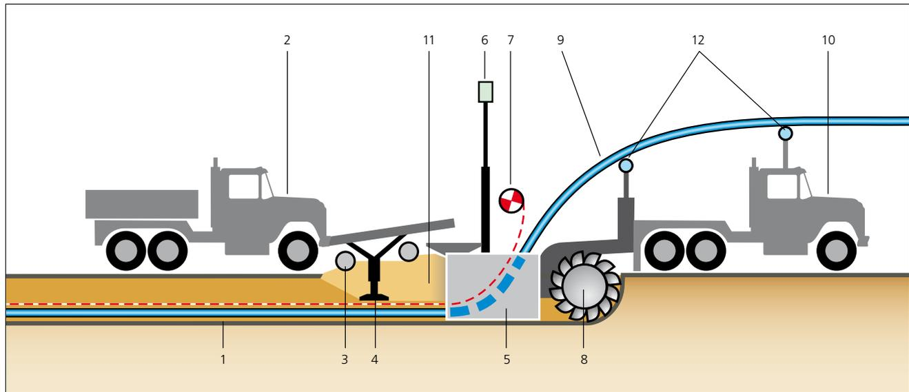
**6.34** Narrow trenching | 1 trench bottom | 2 backfill and compaction unit | 3 axial screw conveyors | 4 compactor | 5 laying box | 6 laser receiver | 7 utility marking tape | 8 milling disc or cutter chain | 9 GEROfit® Rex jacket pipe | 10 trenching and laying unit | 11 extracted material (spoil) | 12 piping guides
