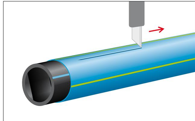
6.11 Surface scratch test acc. to PAS 1075
