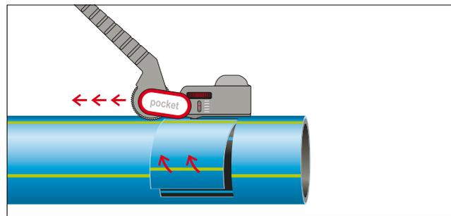
6.87 Cut and strip off the jacket between pipe ends
