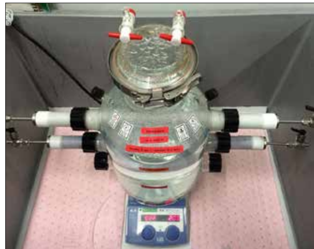
6.5 Permeation test according to KIWA BRL-K 17101
