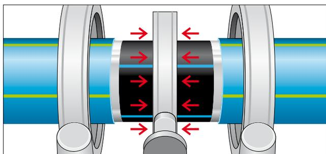
6.56 Initial bead-up and heat soaking
