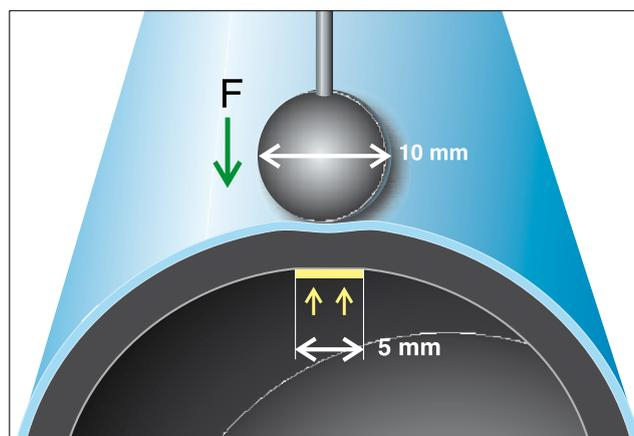
6.9 PLT – Point load test (acc. to PAS 1075)
